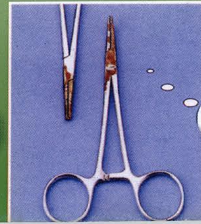
Pitting due to Chlorides
