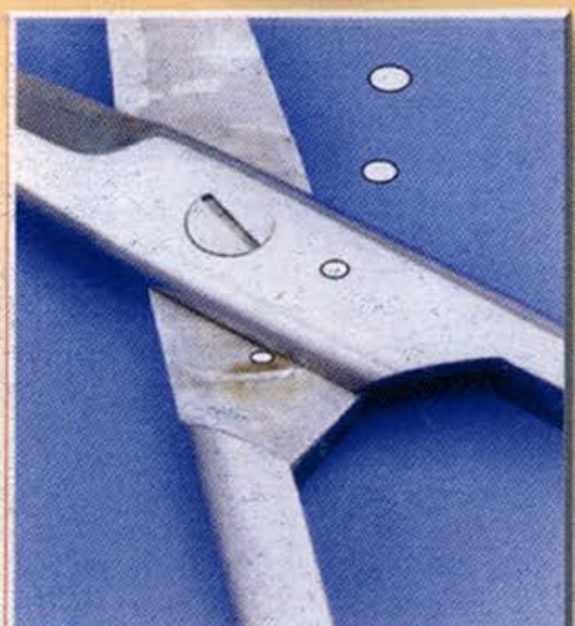
Fretting Corrosion caused due to insufficient treatment with LUBRICATING oil
