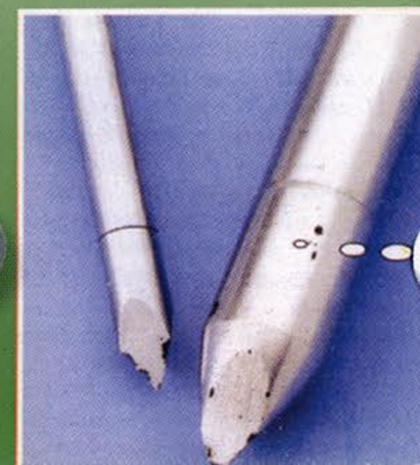
Crevice Corrosion caused due to destruction of natural passive coating of steel due to mechanical / chemical destruction
