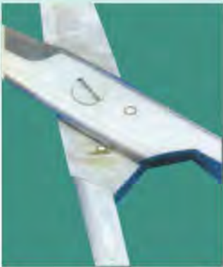
Fretting Corrosion caused due to insufficient treatment with LUBRICATING oil
