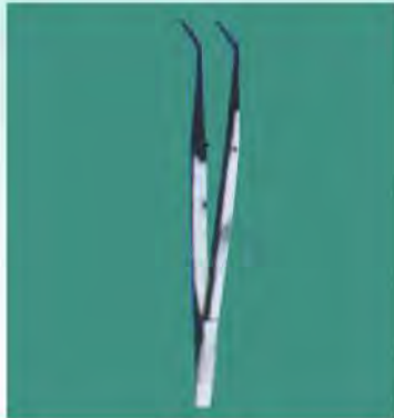
Deposition due to caustic solution containing chlorides
